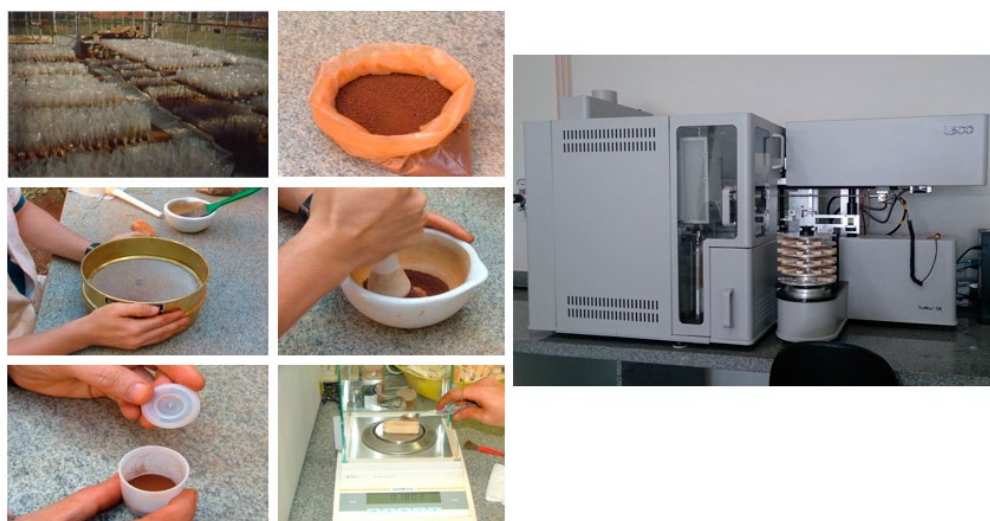
Figure 5.7. Steps for preparing the collected samples (sieving and grinding), weighing and elementary analyzer equipment to determine the C content of the sample.
