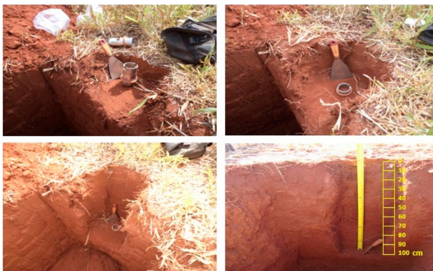
Figure 5.6. Collection of soil samples in trenches 1.5 m deep for sampling up to the 90-100 cm layer.
