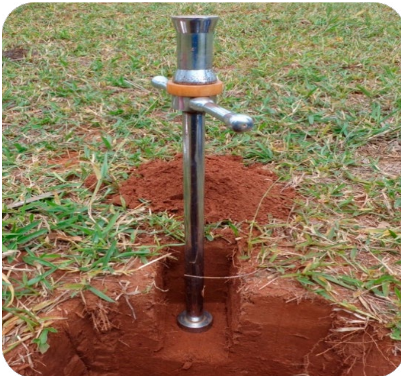
Figure 5.8. Collector auger for undisturbed samples (using volumetric ring) to determine soil bulk density.
